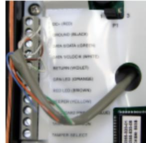
Match the corresponding wire to the screw connector. See pinout table below for additional information.
