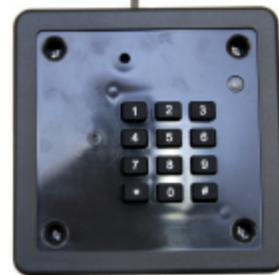
After the front plate has been removed, 4 holes containing screws will be revealed. Remove all 4 screws.
