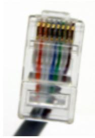
Match the corresponding wire to the appropriate pin on the RJ45 connector. See pinout table below for additional information.
