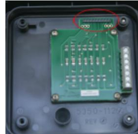
Put the two pieces back together. First, on the inside cover, locate the 10-pin male connector. This connector will need to correspond to the 10-pin female connector on the board on the base unit (image below).
