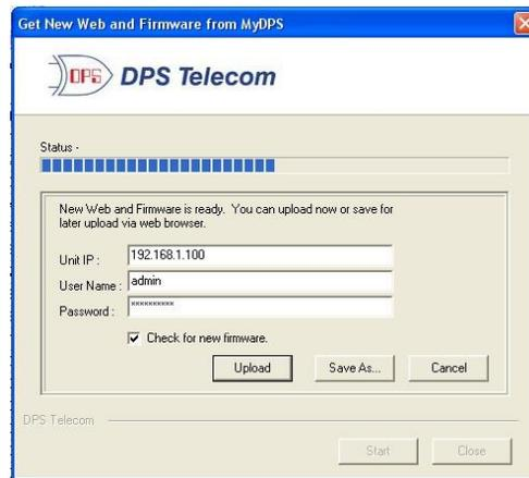
**Fig. 17** Upload New Firmware
