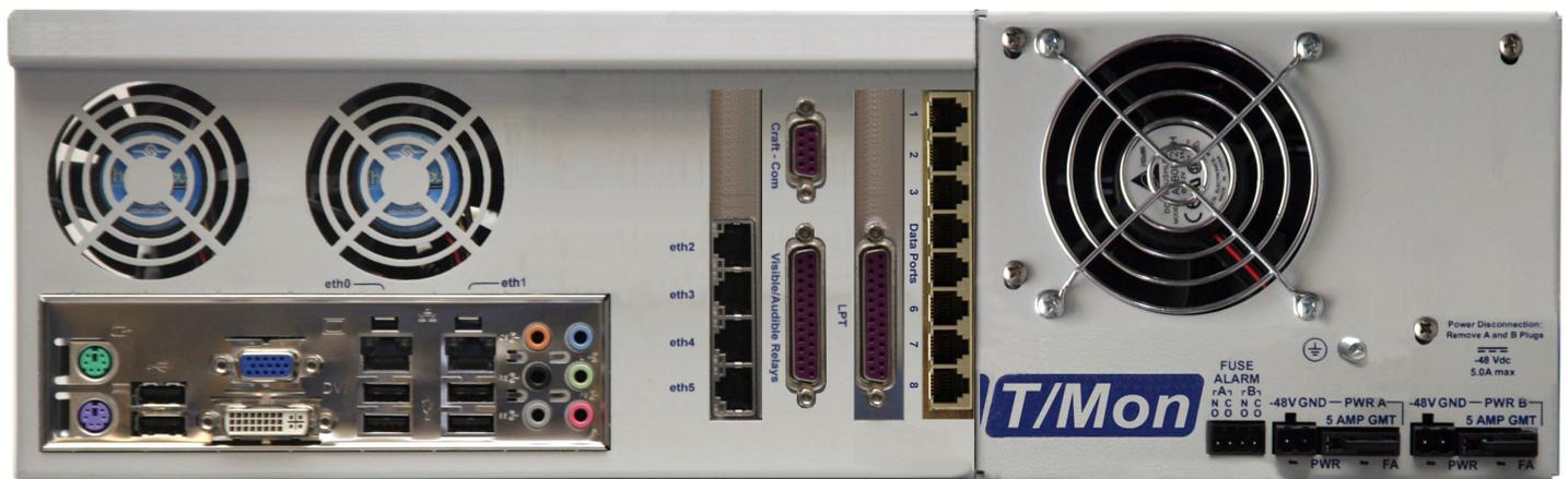
The T/Mon SLIM back panel includes many of the same elements as the T/Mon LNX back panel. T/Mon SLIM is scaled for medium-sized networks with up to 64 devices.
