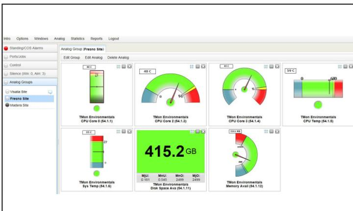
Analog, discrete, and equipment alarms are integrated into the same display. Above are T/Mon Web 3.0 analog gauges.
