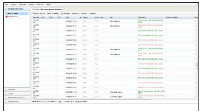
The Standing Alarms screen displays currently failed alarms. The Standing Alarms list is continually updated to reflect the state of the network, giving you an easily accessible list of all current threats to network integrity. Even if the system operator acknowledges the alarm, it remains in the Standing Alarms screen until it is cleared.
