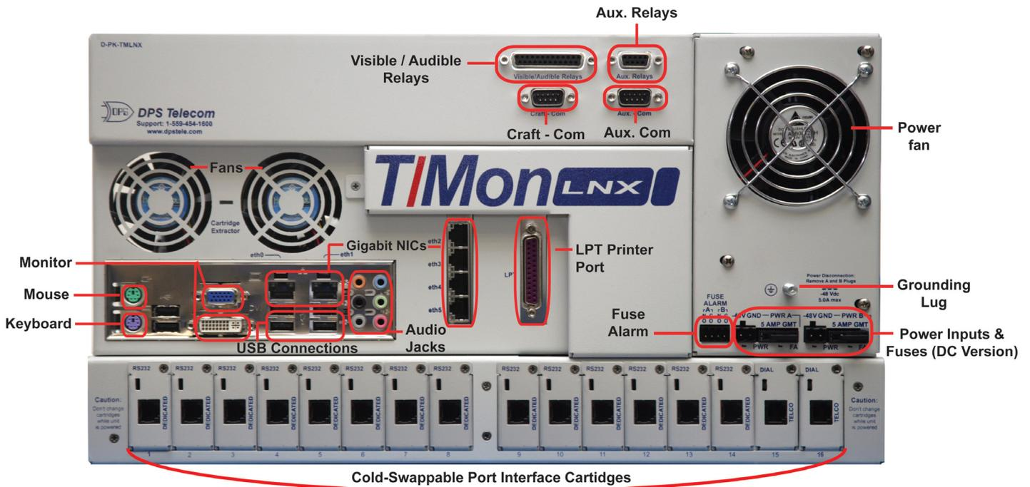
The T/Mon LNX back panel features six 10/100/1000 NICs, up to 16 polling ports, a COM port, a video out port, a fuse alarm port, a POTS line jack, a parallel printer port, a LAN connection port, and dual power feeds.
