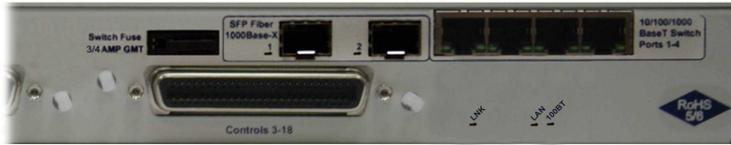
*Back panel (with Fiber Option) LEDs*
