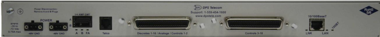
Fig. 5.1 NetGuardian M16 G2 / V16 G2 back panel connections
