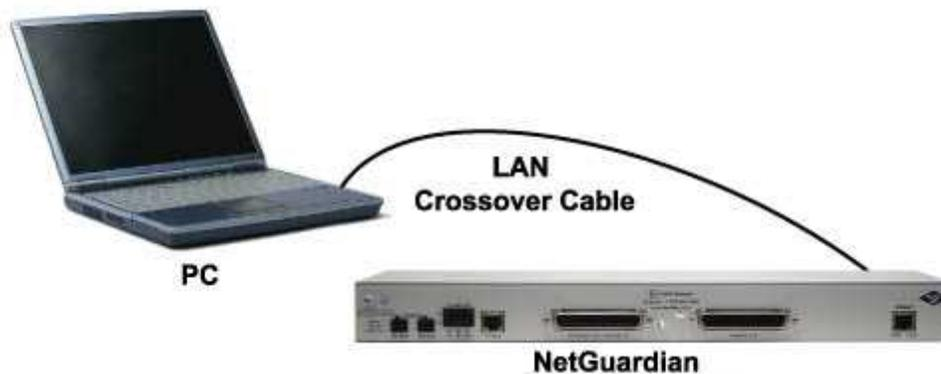
*Fig. 7.1 Connection through Ethernet port*
