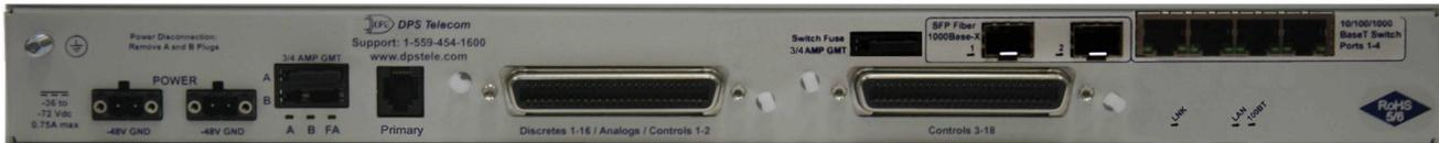
Fig. 5.2 NetGuardian M16 G2 / V16 G2 back panel (with Fiber Option)
