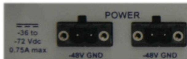
Fig. 5.4 Locking RIA power inputs
