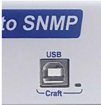
**Fig. 6.2** Modbus Converter Craft Port
