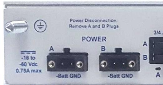
**Fig. 4.3** Modbus Converter Power Terminal
