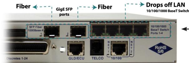
New fiber interface option provides dual SFP fiber ports, in addition to GigE connection.
