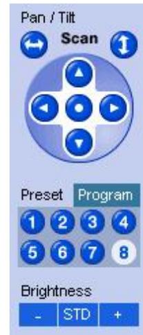
**Fig. 3.11.** Use the arrow buttons to use the pan-and-tilt features of the NetGuardian SiteCAM
