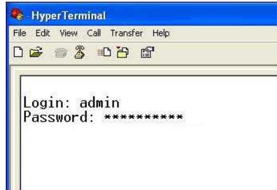
7. The NetGuardian 216 G3's main menu will appear. Type C for C)onfig, then E for E)thernet. Configure the unit's IP address, subnet mask, and default gateway.
