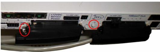
7. Tighten the 2 screws located to the right of the amphenol cables. Use the plastic zip ties provided to secure both cables to the NetGuardian where shown (bottom image). **Note:** A zip tie will be used on the NetGuardian's small metal tab to secure the left amphenol cable. If your remote is equipped with the 4-pin analog connector, connect it to the NetGuardian **and** to the DB9 on the hinged panel.
