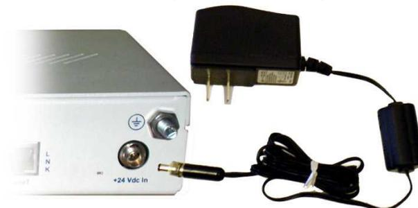
*Fig. 5.3 Close-up view of NetGuardian's screw-on power connector.*
