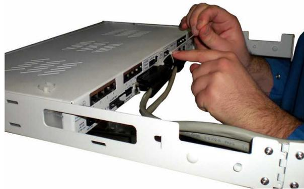
8. Use the remaining zip ties to keep the amphenol cords tied together. Trim the excess plastic off the zip ties with scissors.
