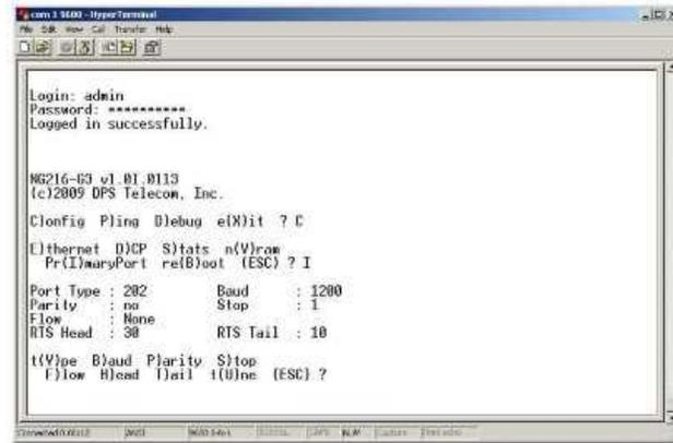
Fig. 8.1 - Serial port configuration
