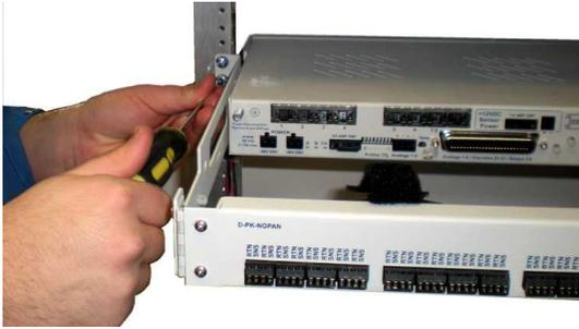
5. Attached the left side of the hinged panel to the rack with the screws provided.
