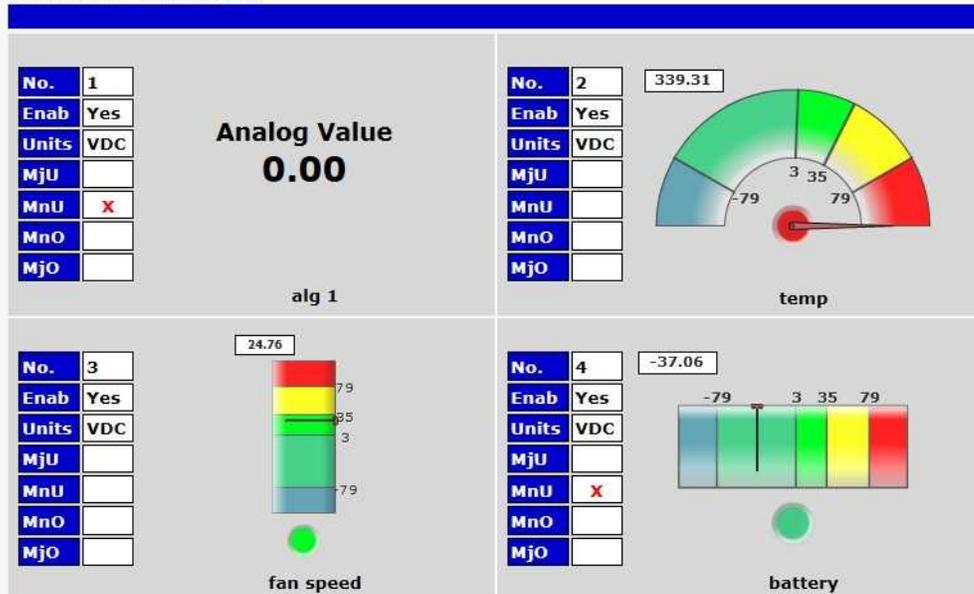
**Fig. 12.6** Current status of all analog inputs in the Monitor > User Analogs in Gauge View.
