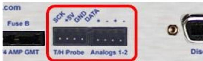
*Fig. 6.5.4.1. Temperature Sensor and Analog Connectors*
