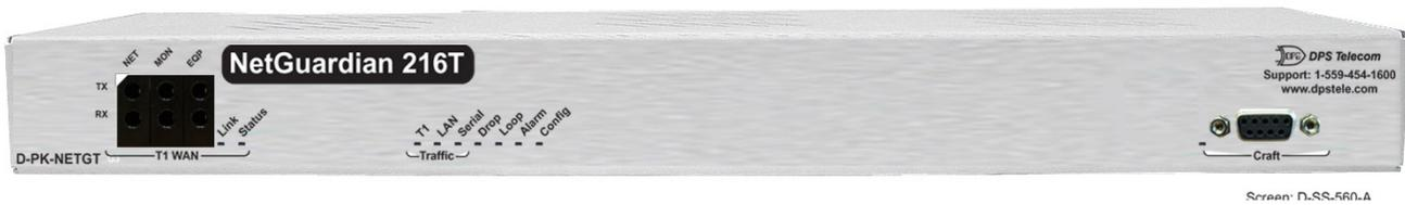
*Fig. 1.1. The NetGuardian 216T monitors alarms, pings network elements, and reports via SNMP, pager, or email*
