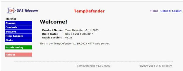
The TempDefender IT features a built-in Web Browser Interface that allows you to manage alarms and configure the unit through the Internet or your Intranet. You can quickly set up alarm point descriptions, view alarm status, issue controls, and configure paging information, and more using most commonly used browsers.
