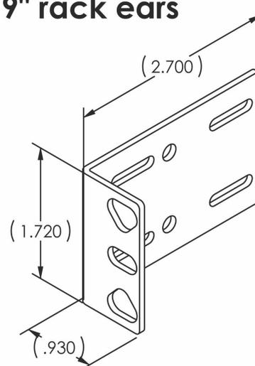
The compact TempDefender IT occupies only half the width of a standard rack unit. Only one rack ear is supplied with the TempDefender IT, and the rack ear can be mounted on the left or right side of the unit. The TempDefender IT mounts in a 19" or 23" rack, and can be mounted on the right or left, in the flush-mount or rear mount locations.
