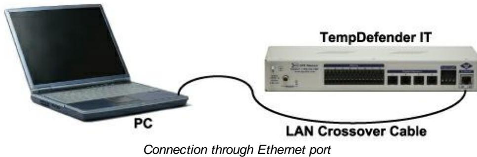
To connect to the TempDefender IT via LAN, all you need is the unit's IP address (Default IP address is 192.168.1.100).
