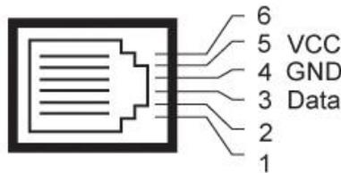
Pinout for the TempDefender and D-Wire Sensor RJ-11 jacks
